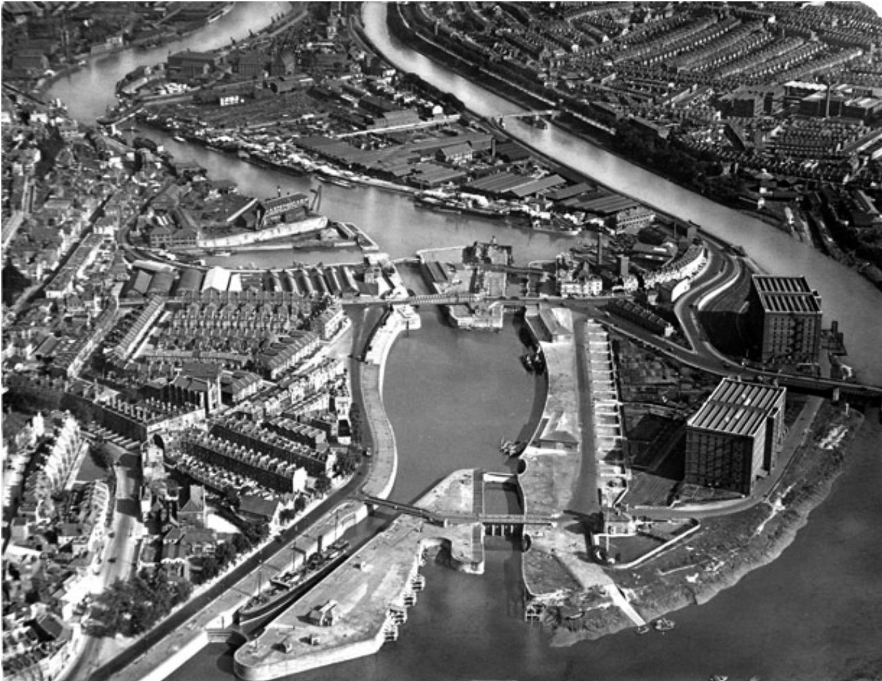
An aerial view of the Floating Harbour and the still tidal New Cut in the 1950's. You can see the timber drying sheds on Baltic Wharf, and Brunel's original swing bridge crossing the lock before the Plimsole Bridge replaced it.
